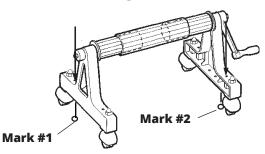
Using one of the two holes in the Frame as a guide make mark #1 on deck. With a 1/2" concrete drill bit, drill a 1 1/2" deep hole at mark #1. Complete steps 6 and 7 before continuing to the other side of the unit. On the other side of the roller unit, make mark #2 by using one of the two holes in the Frame as a guide. With a 1/2" concrete drill bit, drill a 1 1/2" deep hole
