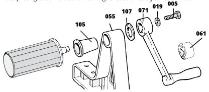
Push the Tube into the Black Bushing then into the Frame. Put the Black Washer over the end of the protruding end of the Hub and slide the Handle onto the end of the Hub.
