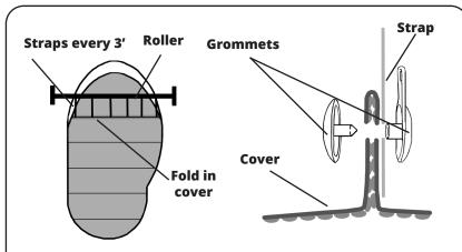
For odd shaped pools, pinch the cover and attach the strap as shown. Attach the cut cover to the roller with the straps (see Grommet detail) by folding the cover in a straight line as shown in the diagrams. Ensure that the fold in the cover is straight.
