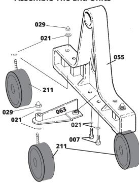
Bolt the Wheels to the Frames and to the 3rd Leg Frame, as shown in the diagram. Next, bolt the 3rd Leg Frames to the Frames.
