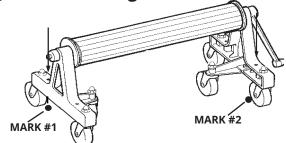
Using one of the two holes in the Frame as a guide, make mark #1 on deck. With a 1/2" concrete drill bit, drill a 1 1/2" deep hole at mark #1. Complete steps 5 and 6 before continuing with step 4. On the other side of the roller unit, make mark #2 by using one of the two holes in the A-frame as a guide. With a 1/2" concrete drill bit, drill a 1 1/2" deep hole at mark #2.
