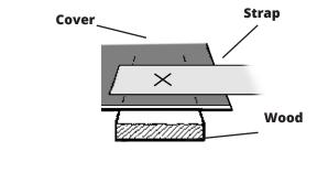
Cross cut through the strapping and the cover. Ensure that the hole in the strapping is at least 1" from the end of the strap and that the hole in the cover is at least 2" from the end of the cover. If possible fold the edge of the cover over so that you put the Grommet through two layers of cover.
