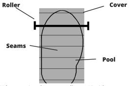
When cutting the cover, allow a 1" wide border around the pool edge to compensate for shrinkage.
