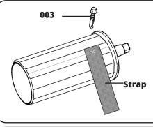
Using 5/8" Tek Screws, secure the strap to the Tube. Make sure you put the screw about an inch into the strap to prevent tearing.
