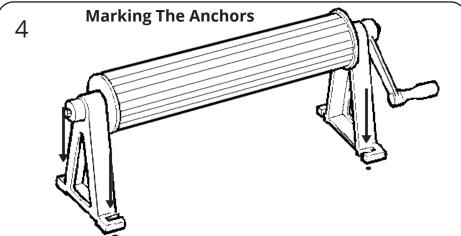
Using the two holes of the Frame as guides, make two marks on the pool deck for each Frame. With a 1/2" concrete drill bit, drill a 1 1/2" deep vertical hole at each mark.
