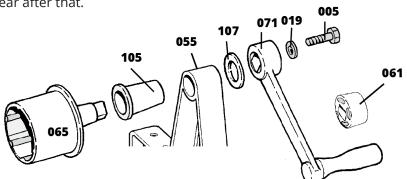
Push the Hub with the Black Bushing into the Frame.
