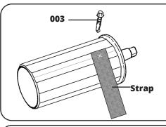
Using 5/8" Tek Screws, secure the strap to the Tube. Make sure you put the screw about an inch into the strap to prevent tearing.
