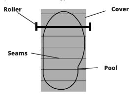
When cutting the cover, allow a 1" wide border around the pool edge to compensate for shrinkage.
