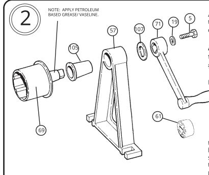
Assemble one end unit to the tube, using the small handle (item #71), as shown in the diagram.
