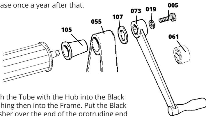
Push the Tube with the Hub into the Black Bushing then into the Frame. Put the Black Washer over the end of the protruding end of the Hub and slide the Handle onto the end of the Hub.
