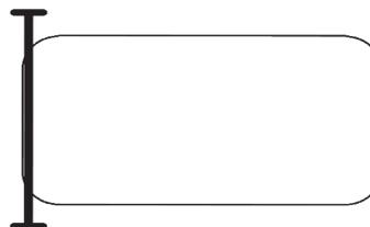
For **irregular** shaped pools, the outside edge of the Tube should be a **minimum** of 3' inside from the end of the pool. Place the reel at the widest point for a better result
