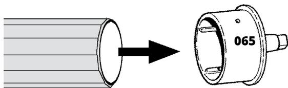
Using two 7/8" TEK Screws (part 001) attach the 4" Hubs to the Tubes.
