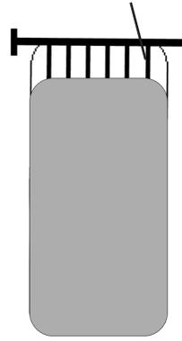
Attach the cut cover to the roller with the blue straps (See grommet detail). Ensure the length of the strap allows the cover to lay flat on pool, to prevent wind from getting under the cover.
