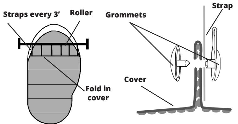
For odd shaped pools, pinch the cover and attach the strap as shown. Attach the cut cover to the roller with the blue straps (see grommet detail) by folding the cover in a straight line as shown in the diagrams. Ensure that the fold in the cover is straight.
