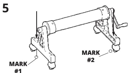
Using one of the two holes in the Frame as a guide, make mark #1 on deck. With a 1/2" concrete drill bit, drill a 1 1/2" deep hole at mark #1. Complete steps 6 and 7 before continuing to the other side of the unit.
