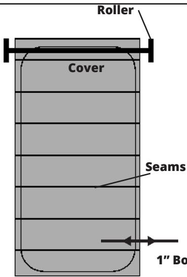
Open the cover over the pool and set it into position. Ensure that the end of the cover (where it attaches to the roller) is square to the roller.
