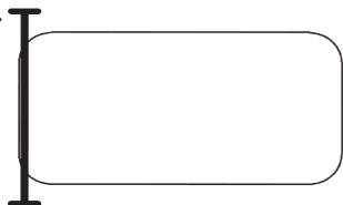
For irregular shaped pools, the outside edge of the Tube should be a minimum of 3' inside from the end of the pool. Place the reel at the widest point for the best result.
