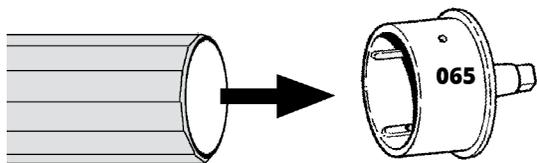
With 2 TEK screws (part 001), attach the Hubs to the Tube using a drill.
