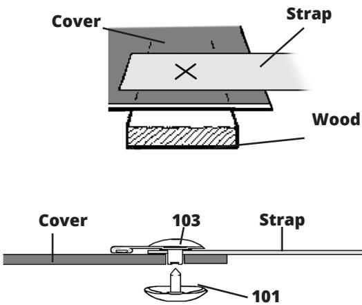
Position the blue strap on the cover. Cross cut through the strapping and the cover. Ensure that the hole in the strapping is at least 1" from the end of the strap and that the hole in the cover is at least 2" from the end of the cover. If possible fold the edge of the cover over so that you put the Grommet through two layers of cover.
