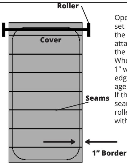
Open the cover over the pool and set it into position. Ensure that the end of the cover (where it attaches to the roller) is square to the roller.
