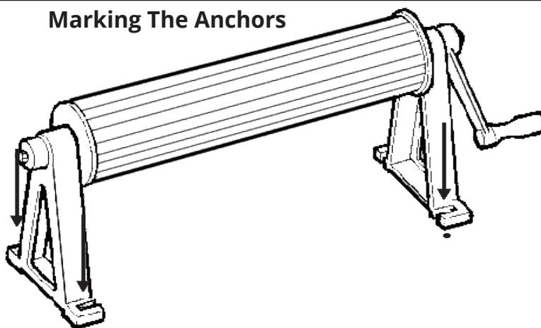
Using the two holes of the Frame as guides, make two marks on the pool deck for each Frame. With a 1/2" concrete drill bit, drill a 1 1/2" deep vertical hole at each mark.
