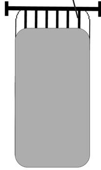
Attach the cut cover to the roller with the blue straps (see Grommet detail). Ensure the length of the strap allows the cover to lay flat on pool, to prevent wind from getting under the cover.
