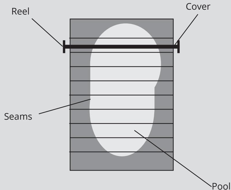
When cutting the cover, allow a 1 1/2" wide border around the pool edge to compensate for shrinkage.
