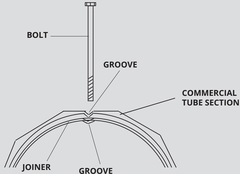
It is very important that you ensure the groove of the joiner is right under the groove of the commercial tube.
