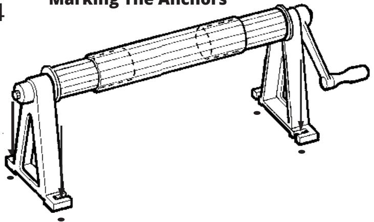
Using the two holes of the #4 A-frame (item #57) as guides, make two marks on deck for each #4 A-frame. With a 1/2" concrete drill bit, drill a 1 1/2" deep vertical hole at each mark.
