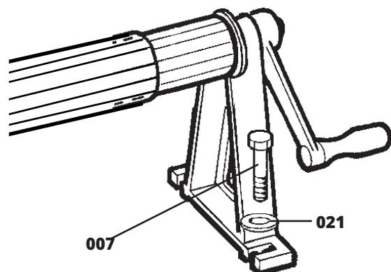
Open the cover over the pool and set it into position. Ensure that the end of the cover (where it attaches to the roller) is square to the roller.
