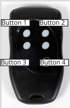
5. If you want the buttons to be reversed repeat steps 2 and 3 but press and hold Button 3 instead of 1. This can be useful if you are programming multiple motors work in unison.
