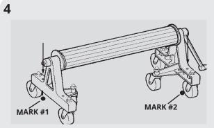
Using one of the two holes in the Frame as a guide, make mark #1 on deck. With a 1/2" concrete drill bit, drill a 1 1/2" deep hole at mark #1. Complete steps 5 and 6 before continuing with step 4. On the other side of the roller unit, make mark #2 by using one of the two holes in the A-frame as a guide. With a 1/2" concrete drill bit, drill a 1 1/2" deep hole at mark #2.
