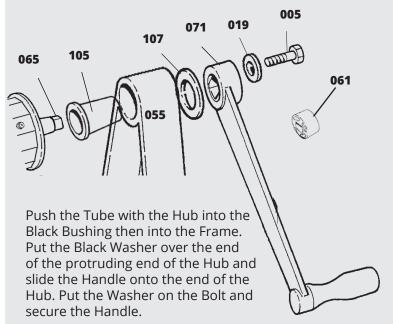
**NOTE** do not overtighten this Bolt as it will make it hard to rotate the Handle.
