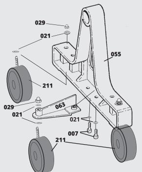
Bolt the Castors to the Frames and to the 3rd Leg Frame, as shown in the diagram. Next, bolt the 3rd Leg Frames to the Frames.
