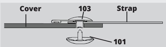
Insert the Female Grommet through your cut in the strapping and the cover. Ensure that the material is completely pushed down on the shaft. Insert the Male Grommet into Female Grommet. Once in place, hit with a hammer until secure. (**Caution - excessive force will break grommet**).
