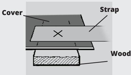
Position the blue strap on the cover. Cross cut through the strapping and the cover. Ensure that the hole in the strapping is at least 1" from the end of the strap and that the hole in the cover is at least 2" from the end of the cover. If possible fold the edge of the cover over so that you put the Grommet through two layers of cover.
