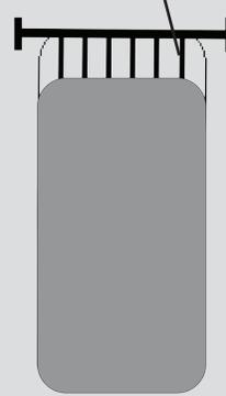
Attach the cut cover to the roller with the blue straps (See Grommet detail). Ensure the length of the strap allows the cover to lay flat on pool, to prevent wind from getting under the cover.
