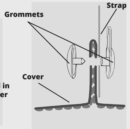
For odd shaped pools, pinch the cover and attach the strap as shown. Attach the cut cover to the roller with the blue straps (see Grommet detail) by folding the cover in a straight line as shown in the diagrams. Ensure that the fold in the cover is straight.
