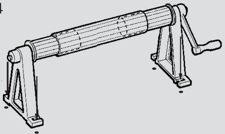
Using the two holes of the #4 A-frame (item #57) as guides, make two marks on deck for each #4 A-frame. With a 1/2" concrete drill bit, drill a 1 1/2" deep verticle hole at each mark.
