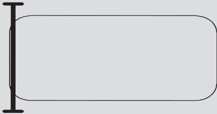
For irregular shaped pools, the outside edge of the Tube should be a minimum of 3' inside from the end of the pool. Place the reel at the widest point if that is possible for a better result.
