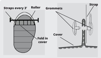
For odd shaped pools, pinch the cover and attach the strap as shown. Attach the cut cover to the roller with the blue straps (see grommet detail) by folding the cover in a straight line as shown in the diagrams. Ensure that the fold in the cover is straight.
