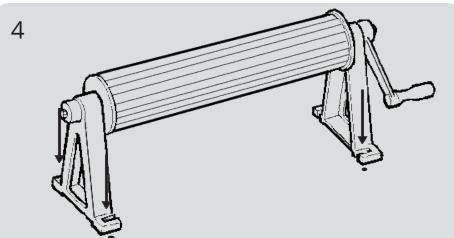
Using the two holes of the Frame as guides, make two marks on the pool deck for each Frame. With a 1/2" concrete drill bit, drill a 1 1/2" deep verticle hole at each mark.
