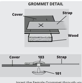
Position the blue strap on the cover. Cross cut through the strapping and the cover. Ensure that the hole in the strapping is at least 1" from the end of the strap and that the hole in the cover is at least 2" from the end of the cover. If possible fold the edge of the cover over so that you put the Grommet through two layers of cover.
