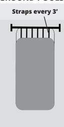
Attach the cut cover to the roller with the blue straps (see Grommet detail). Ensure the length of the strap allows the cover to lay flat on pool, to prevent wind from getting under the cover.
