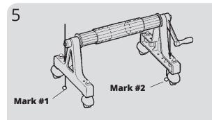
Using one of the two holes in the Frame as a guide make mark #1 on deck. With a 1/2" concrete drill bit, drill a 1 1/2" deep hole at mark #1. Complete steps 6 and 7 before continuing to the other side of the unit. On the other side of the roller unit, make mark #2 by using one of the two holes in the Frame as a guide. With a 1/2" concrete drill bit, drill a 1 1/2" deep hole at mark #2.
