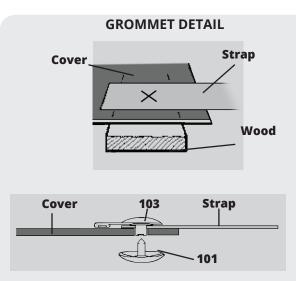
Position the blue strap on the cover. Cross cut through the strapping and the cover. Ensure that the hole in the strapping is at least 1" from the end of the strap and that the hole in the cover is at least 2" from the end of the cover. If possible fold the edge of the cover over so that you put the Grommet through two layers of cover.
