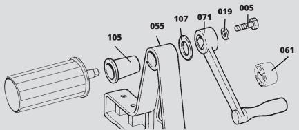
Push the Tube into the Black Bushing then into the Frame.
