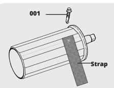
Using Tek Screws, secure the strap to the Tube. Make sure you put the screw about an inch into the strap to prevent tearing.
