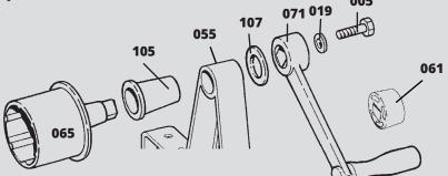
Push the Hub with the Black Bushing into the Frame. Put the Black Washer over the end of the protruding end of the Hub and slide the Handle onto the end of the Hub.
